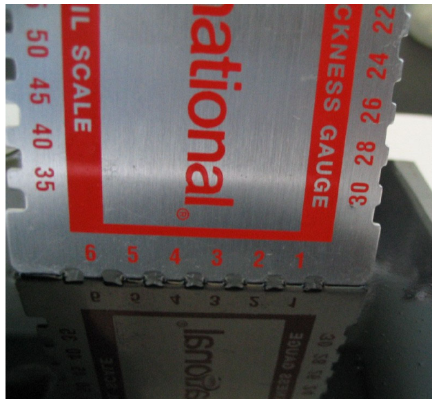
Figure 4. WFT Gauge Positioned in Wet Paint Film.
